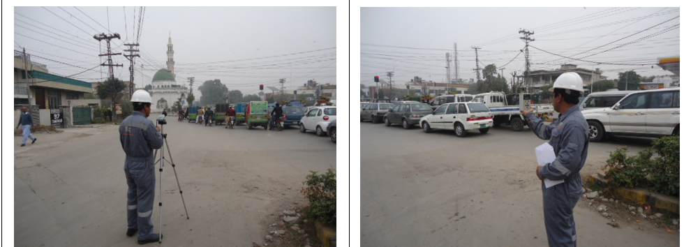
Particulate Matter & Noise Level Monitoring
